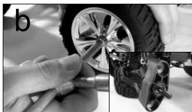
a. Insert the wheel hex adapter into both sides of the front / rear wheel.
