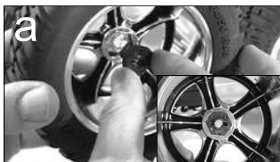
a. Insert the wheel hex adapter into both sides of the front / rear wheel.
