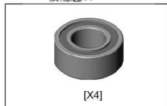
PD1968 B. BEARING (4), d5*D10*W4 滾珠軸承(HMV1050LLY)
