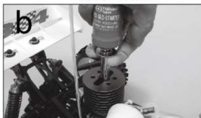
c. Pull on the engine starter, release, repeat until the engine starts. Throttle maybe required to be opened momentarily, but release back to neutral immediately after it starts.
