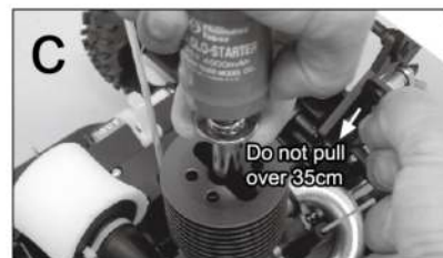
c. Pull on the engine starter, release, repeat until the engine starts. Throttle maybe required to be opened momentarily, but release back to neutral immediately after it starts.
