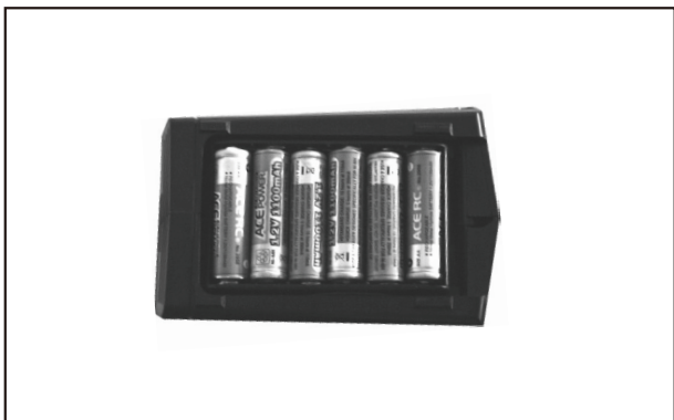
3. Install 6 AA dry-cell batteries. (not included) Note the battery polarity order.
